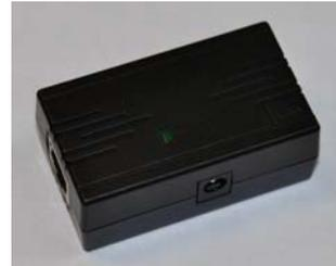
There are two RJ45 connectors on a power injector. Please ensure that the outdoor ZipLink radio Ethernet cable gets plugged into the side that says "PoE". This stands for "Power over Ethernet" and is how the radio unit gets power. The Ethernet jack on the other side labeled "LAN" will connect to your laptop, Ethernet switch or equipment. The round barrel connector is where the power adaptor connects.
