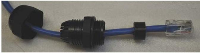
The next step is to push the rubber ring into position so that it will compress when the gland is assembled. You should GENTLY use a small screwdriver to slide it inside the main body of the gland housing until it is flush with the little plastic fingers at the bottom of the gland, like shown in the picture to the right:
